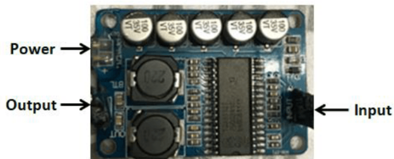
Figure 5.3: View of the current amplifier (TDA 8932).
