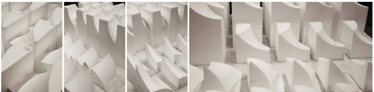
Figure 4.40. Gyroid fundamental patches cut from EPS blocks
