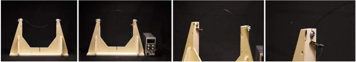
Figure 3.27. Hotwire cutter tool frame and power supply
