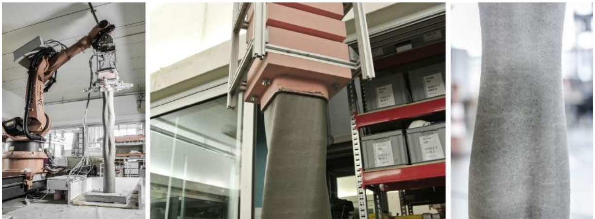
Figure 1.5. Smart Dynamic Casting, ETH Zürich, 2012-2015 (URL-23)
