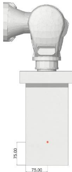
Figure 4.5. TCP position of the experiment#1. Dimensions are in mm
