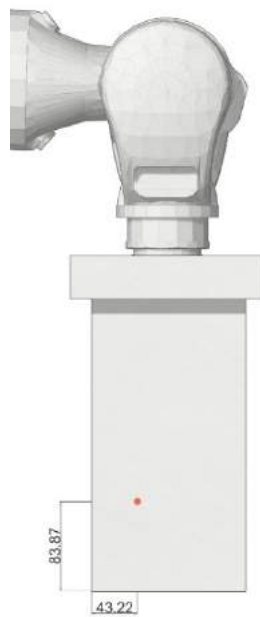
Figure 4.13. TCP position of the experiment#2. Dimensions are in mm
