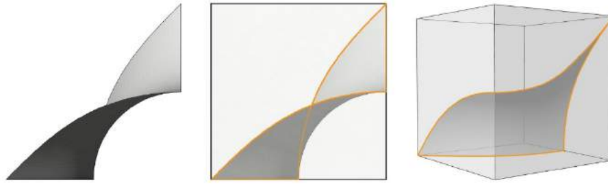
Figure 3.12. Edge curves of the Gyroid fundamental patch
