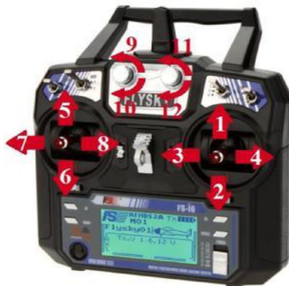
Figure 4.4 Channels and actions on remote controller
