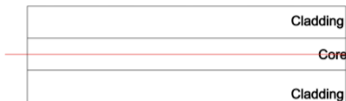
Figure 2.8. Schematics of single mode fiber
