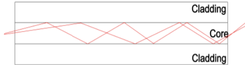
Figure 2.9. Schematics of step index multi mode fiber
