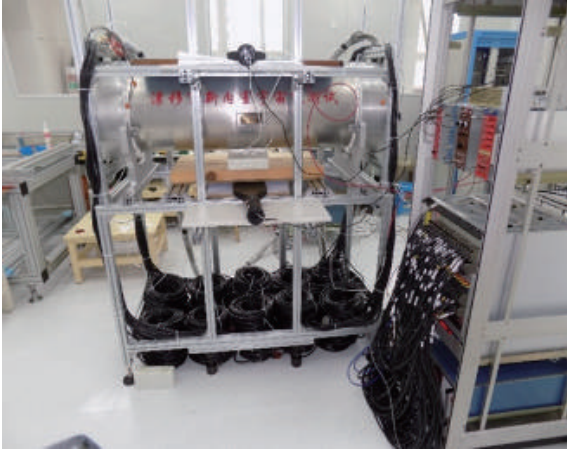
Fig. 1.12. (color online) The cosmic-ray test of the new inner MDC.
