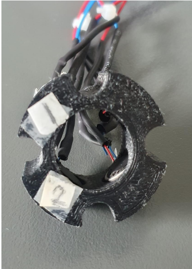
Figure 11: Final ring after 3D printing
